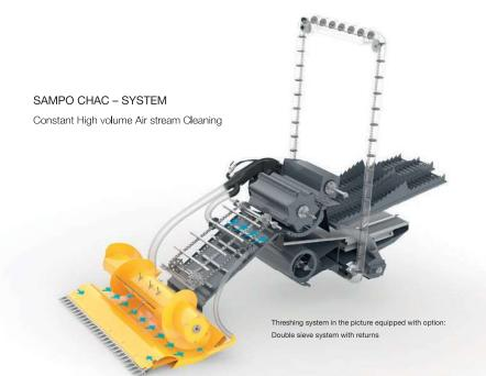
The C2 is equipped with three straw walkers and a single sieve system. The walker area is easy to access from a hatch from the rear. For additional efficiency an optional double sieve system can be fitted on the combine. With the added sieve area, you can choose between 5 different sieves, 5,8,10,12 or 16 mm. The upper sieve is adjustable. This system includes also an efficient return system. The returns are blown back to the grain pan area.
